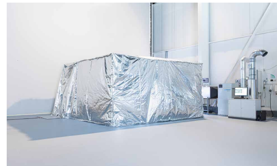
DryClean-CAPE® for dry-room testing; Source: Fraunhofer Institute for Manufacturing Engineering and Automation IPA
