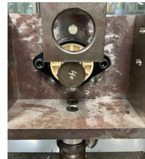
Pressure test on our compact two hole flange bearing.
