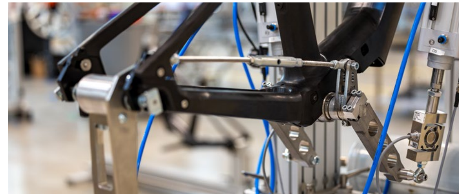
The injection moulded frame on the test rig in our test laboratory.
