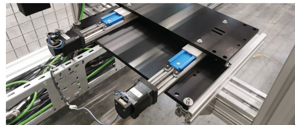
In the endurance test: Two NTM-45 systems in horizontal installation position System length 200mm, speed 0.015m/s
