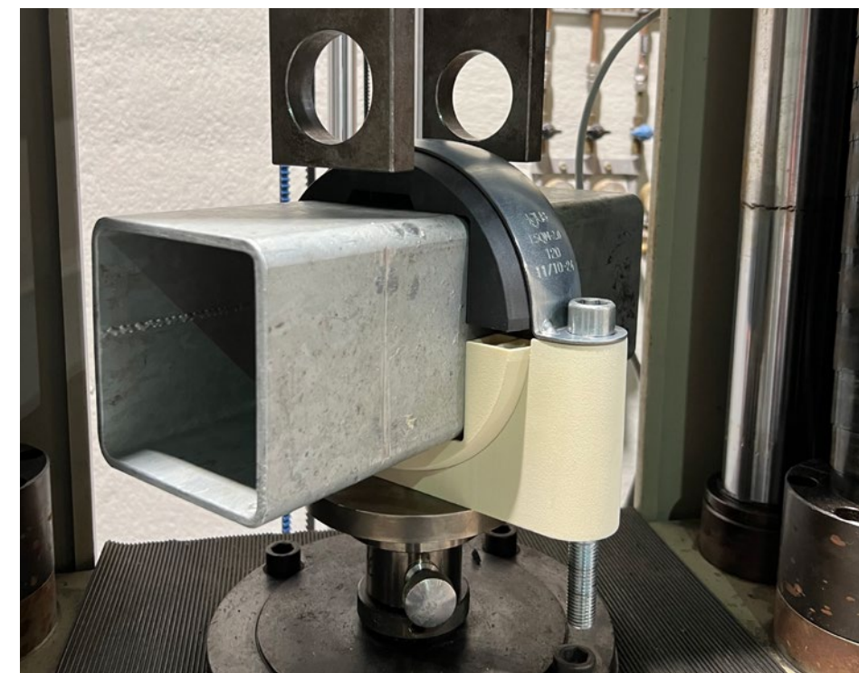
3D-printed prototype of the ESQM-2.0-120-HD put to the test.
