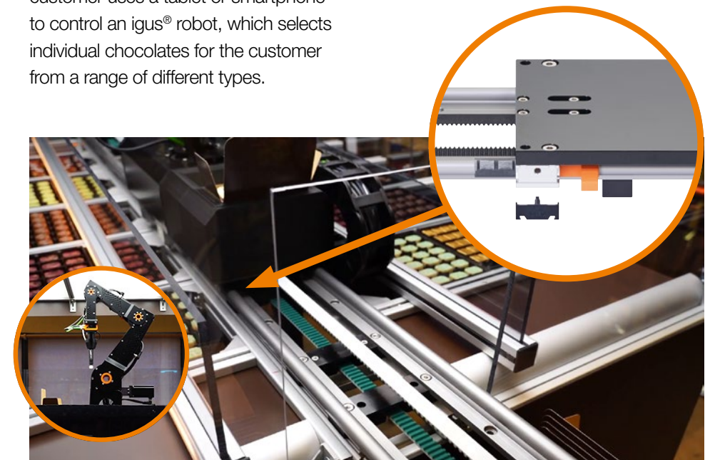
Exchange bearing in the 7th robot axis
