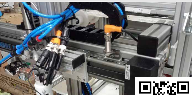
In the video: An automatic labelling machine, consisting of a drylin® room linear robot, labels farmhouse ice cream.
