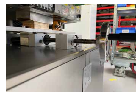
Station adjustment below the labeller using drylin® linear technology.
