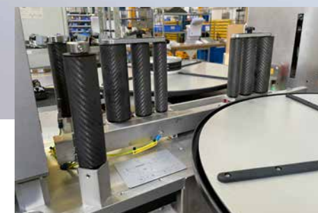
Lightweight guide rollers with xiros® ball bearings guide the labels into the labeller.
