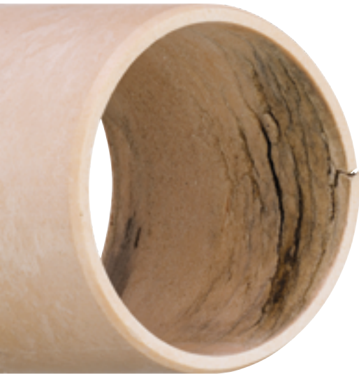
Damage due to permanent overload (Source: igus®)
