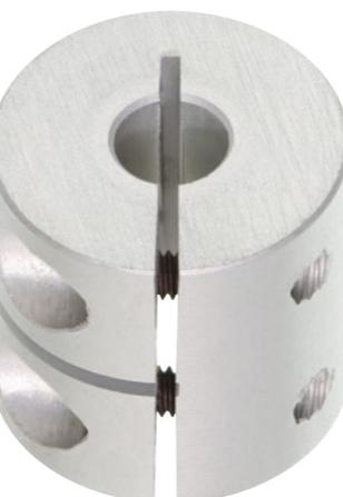
The shaft coupling transmits torque between two shafts, such as a lead screw linear unit and a motor. The cost-effective and space-saving aluminium couplings are mainly used in miniature drive technology. The rigid coupling can absorb both axial and radial forces.
