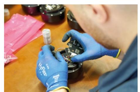
Equipping the axes with circuit boards
