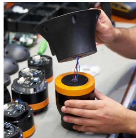
Cables are laid through the gearboxes
