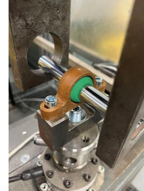
The KSTM-CL-ECO pillow block bearing in a tensile test.
