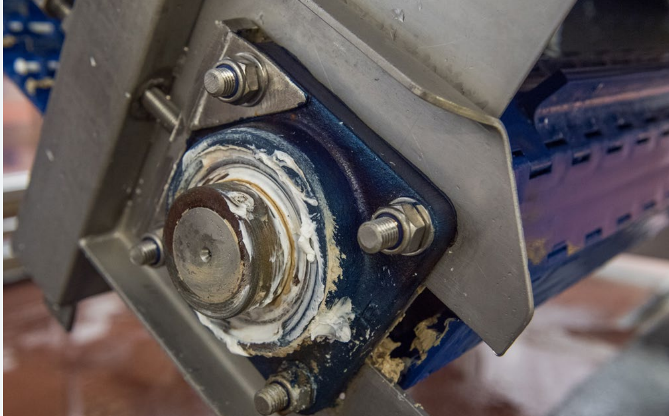
Excess grease from the bearing has collected on the hygienic conveyor belt, increasing the potential for bacteria or allergens to enter the food zone and compromise food safety.
