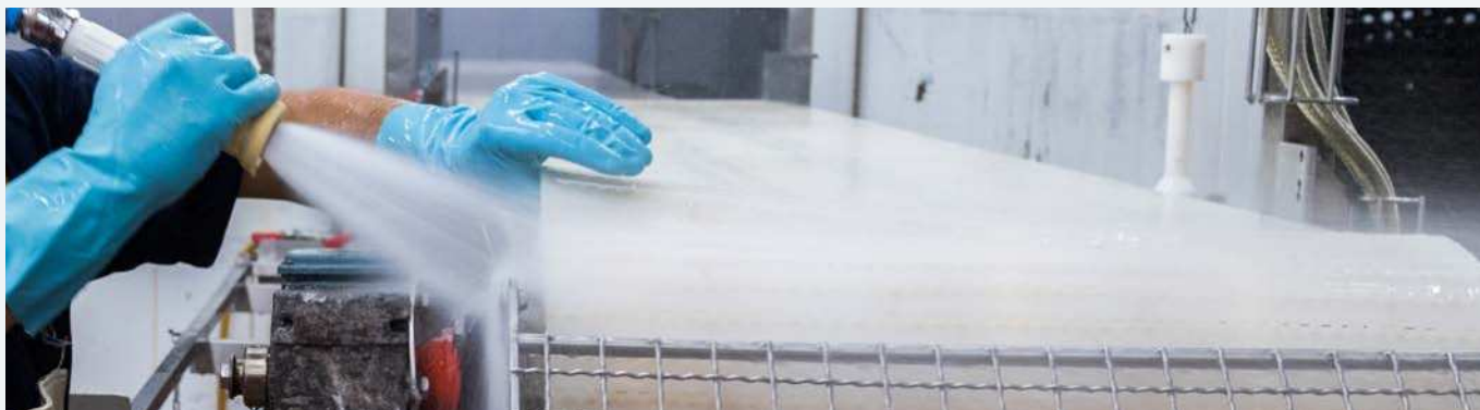
With the SKF solution, the risk of infected bearing grease spreading to the food zone during pressure wash is reduced.
